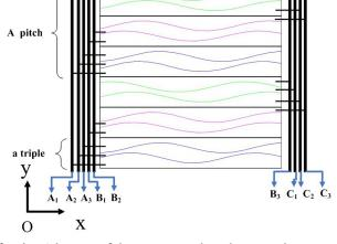
Fig. 1. Schematic of the Vernier anode with two pitches.
