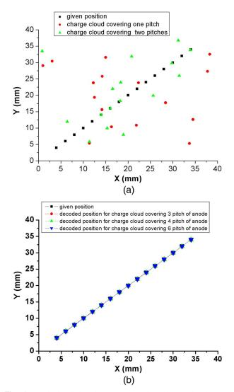
**Fig. 2.** Calculated decoding position when charge cloud covers (a) one to two pitches and (b) no fewer than three pitches for a group of given positions.
