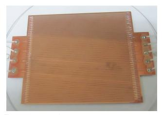
Fig. 7. Photograph of a 38 mm × 38 mm Vernier anode made in copper film on a quartz substrate.
