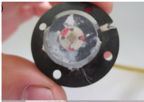
Figure 4. The end surface of the fiber array before being grinded and polished.
