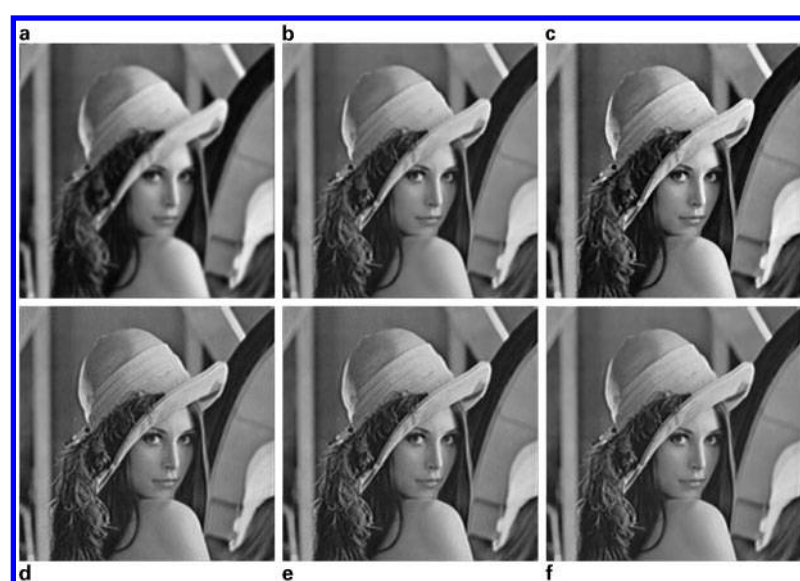
5 Image deblurring experiment with a 512 \times 512 Lena image: a blurred image; b ForWaRD, ISNR=2.34; c FTVd result, ISNR=2.61; d ShearDec result, ISNR=2.73; e L0-Abs result, ISNR=2.87; f our final result, ISNR=3.08
