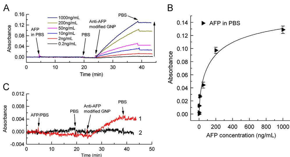
**Fig. 5.** (A) Absorbance response of a 1.0  $\mu$ m OMF to different AFP concentrations in PBS buffer using sandwich assays. (B) Calibration curve of the biosensor as a function of analyte target concentration in PBS. (C) Control experiments: curve 1 represents injection of 1% (v/v) secondary antibody functionalized GNPs solution in the presence of 0.2 ng/mL AFP; curve 2 represents injection of 1% (v/v) secondary antibody functionalized GNPs solution in the absence of AFP.
