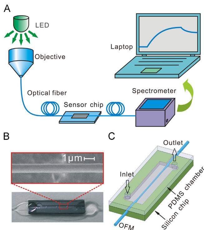
**Fig. 1.** (A) Illustration of the experimental setup. (B) Image of a sensor cell and SEM image of a 1.0  $\mu\text{m}$  thick optical microfiber. (C) Schematic diagram of an OFM sensor device with an integrated PDMS chamber for sample delivery.
