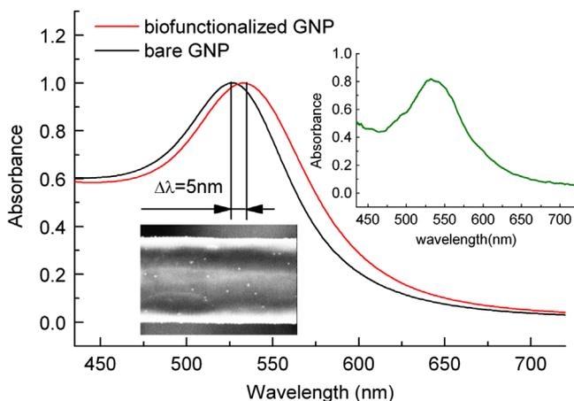
**Fig. 4.** Absorption spectra of GNP solution and biofunctionalized GNP solution with diameter of 40 nm measured by Lambda 850. The insets show the absorption spectra of the secondary antibody functionalized GNPs binding to an AFP coated OMF sensor and a SEM image of the fiber decorated with GNPs.
