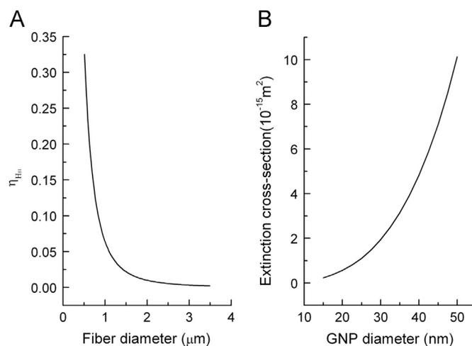
**Fig. 3.** (A) Fraction of  $HE_{11}$  modal power in the external of an OMFs at 520 nm wavelength. The RI of the medium and OMF are 1.333 and 1.450, respectively. (B) Extinction cross-section of gold nanoparticles at the wavelength of their absorption peaks.
