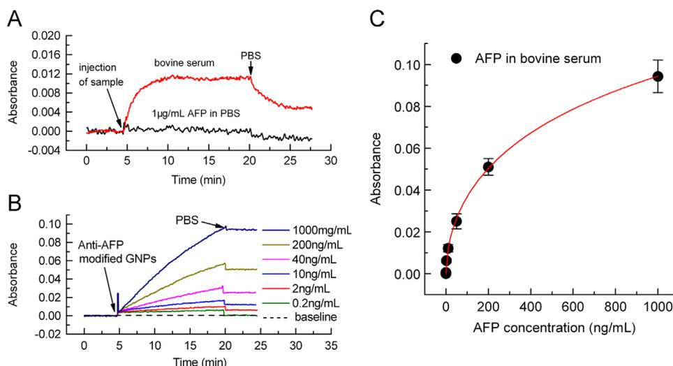
**Fig. 6.** (A) Absorbance responses of the OMF sensor to 1 µg/mL AFP in PBS and bovine serum without AFP, respectively. (B) Secondary antibody functionalized GNP enhanced sensor response to bovine serum samples spiked with different concentrations of AFP. (C) Calibration curve of the biosensor as a function of analyte target concentration in bovine serum.
