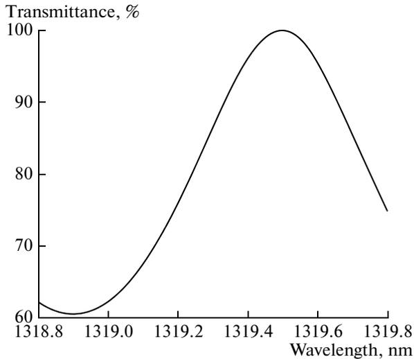
Fig. 4. Transmissivity of etalon around 1319 nm.
