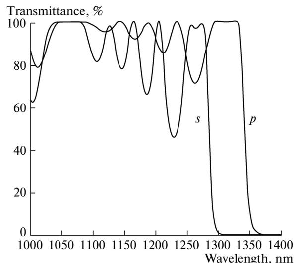
**Fig. 3.** Transmissivity of S2 side of M3,  $s$ - and  $p$ -polarizations.
