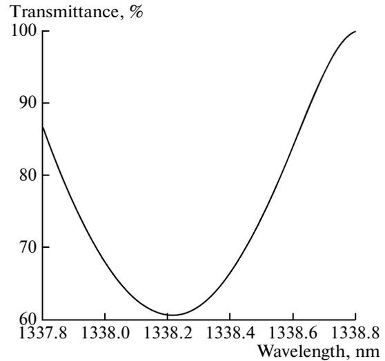
Fig. 5. Transmissivity of 0.8 mm etalon around 1338 nm.
