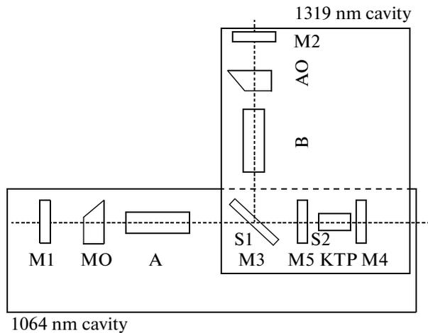
**Fig. 1.** Schematic for the intracavity sum-frequency 589 nm Nd:YAG/KTP yellow laser.
