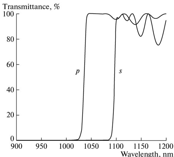
**Fig. 2.** Transmissivity of S1 side of M3,  $s$ - and  $p$ -polarizations.
