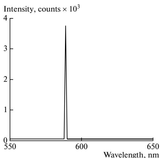
Fig. 8. Spectrum of the output laser at 589 nm.
