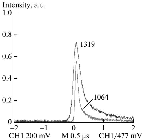
Fig. 6. Temporal profile of two synchronous laser pulses at 1064 and 1319 nm.
