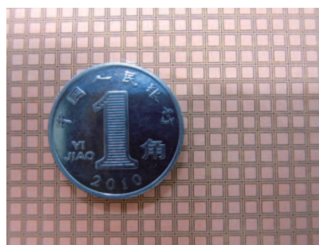
Fig. 8. (color online) The FSS fabricated using standard lithography.
