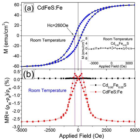
FIG. 4. (Color online) (a) Magnetization of the Fe–CdFeS granular film at room temperature with magnetic field perpendicular to the surface of the sample. The inset shows the  $M$ - $H$  curve of the CdFeS DMS sample at room temperature. (b) Magnetoresistances of Fe–CdFeS granular film and CdFeS DMS thin film at room temperature.
