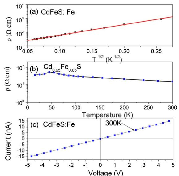
FIG. 3. (Color online) (a) Resistivity  $\rho$  in a logarithmic scale vs  $T^{-1/2}$  for sample A. (b) Temperature dependent resistivity of sample B. (c) Current-voltage curves of sample A measured at room temperature.
