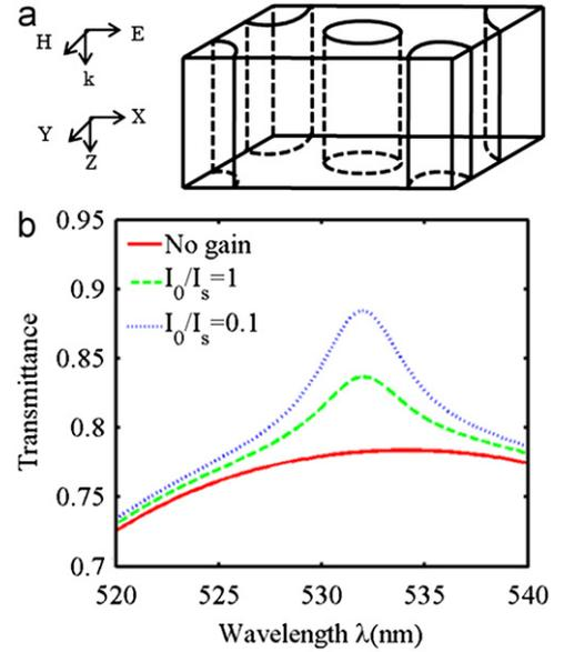
Fig. 5. (a) Basic structural unit in simulation. The slice thickness is 500 nm. Periodic boundary condition is used. (b) The transmittance for without and with gain ( $\chi_{max} = -0.03$ ). Structure parameters are  $a = 40$  nm,  $r = 10$  nm.
