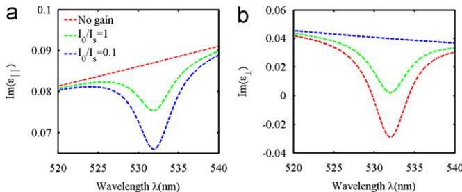
Fig. 4. The imaginary parts of  $\epsilon_{||}$  and  $\epsilon_{\perp}$  for the sample without and with gain ( $\chi_{max} = -0.03$ ) around center frequency  $v_0 = 5.639 \times 10^{14}$  Hz (wavelength  $\lambda = 532$  nm).
