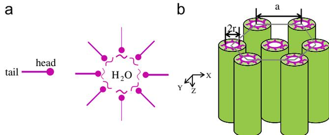
**Fig. 1.** (a) Schematic diagram of amphiphilic molecule hexagonal structure. (b) The RHLLC template structure.  $a$  is the distance of adjacent nanoholes and  $r$  is the radius of nanoholes.
