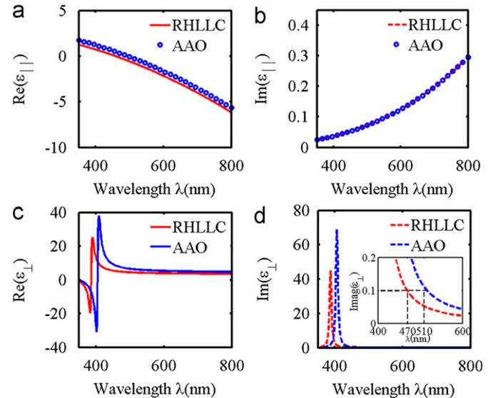
**Fig. 2.** Effective anisotropic permittivities for silver-RHLLC metamaterial and silver-AAO metamaterial. (a) and (b) Real part and imaginary part of  $\epsilon_{\parallel}$ . (c) and (d) Real part and imaginary part of  $\epsilon_{\perp}$ . The inset in (d) is the magnified part in the range  $\lambda = 400\text{--}600 \text{ nm}$ .
