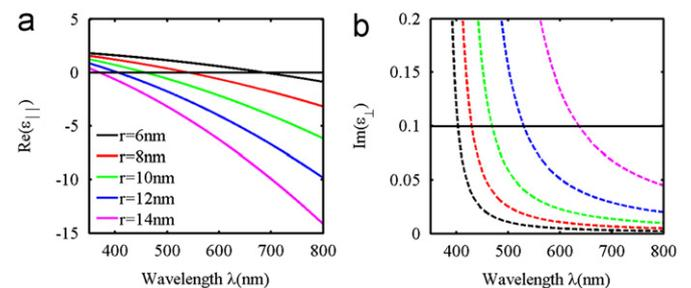
**Fig. 3.** Real parts of  $\epsilon_{\parallel}$  and imaginary parts of  $\epsilon_{\perp}$  for different radii of silver nanowires.
