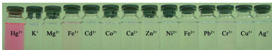
Fig. 1. Visual color changes of RHO (10 \mu\text{M} ) with addition of 5 equiv. of different metal ions in ethanol/water (7:3, v/v), from left to right, the sequence of ions added were \text{Hg}^{2+} , \text{K}^+ , \text{Mg}^{2+} , \text{Fe}^{3+} , \text{Cd}^{2+} , \text{Co}^{2+} , \text{Ca}^{2+} , \text{Zn}^{2+} , \text{Ni}^{2+} , \text{Fe}^{2+} , \text{Pb}^{2+} , \text{Cr}^{3+} , \text{Cu}^{2+} and \text{Ag}^+ .
