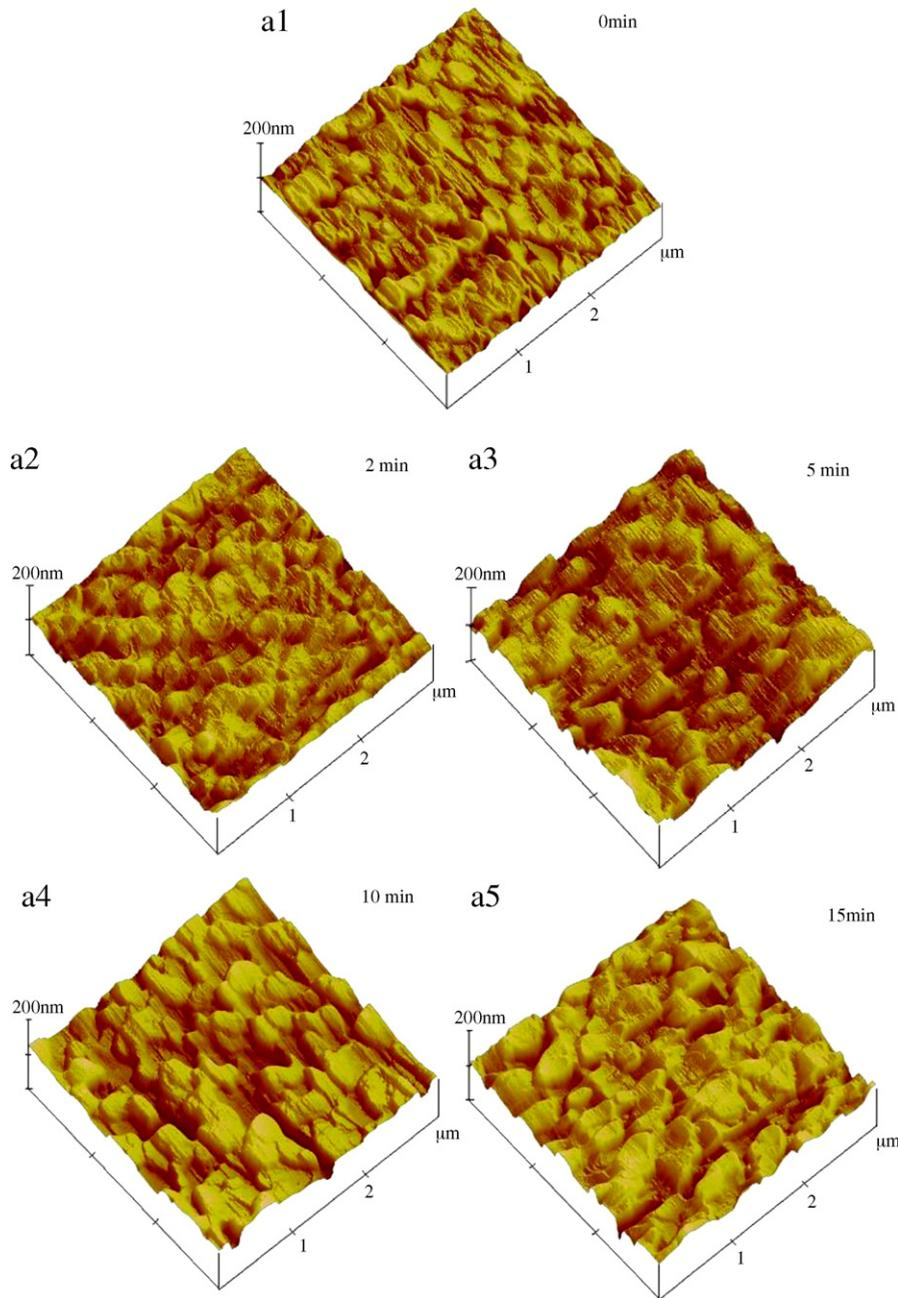
**Fig. 4.** AFM images of  $\text{In}_{0.82}\text{Ga}_{0.18}\text{As}$  buffer layers over an area ( $3 \times 3 \mu\text{m}^2$ ): (a1) as-grown, (a2) thermal annealing for 2 min, (a3) thermal annealing for 5 min, (a4) thermal annealing for 10 min, and (a5) thermal annealing for 15 min.
