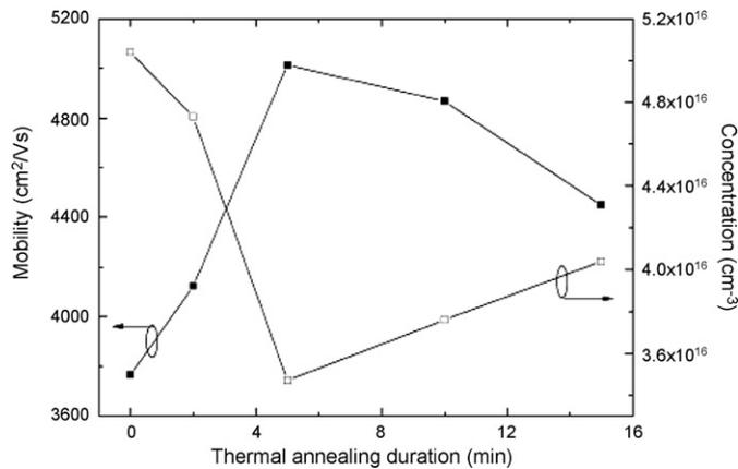
**Fig. 1.** The Hall mobility and carrier concentration measured at room temperature as a function of the buffer layer thermal annealing duration.
