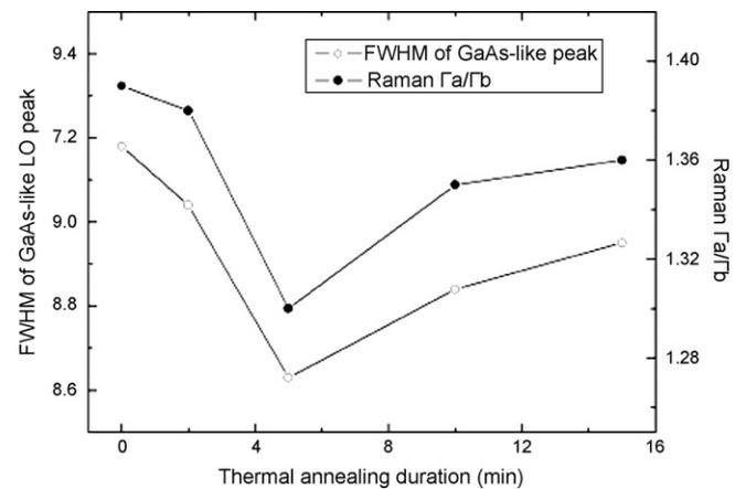
**Fig. 3.** The FWHM of GaAs-like LO peak and asymmetry ratio ( $\Gamma_a/\Gamma_b$ ) of samples  $A_1$ ,  $A_2$ ,  $A_3$ ,  $A_4$  and  $A_5$  with different thermal annealing duration of the  $\text{In}_{0.82}\text{Ga}_{0.18}\text{As}$  epilayers.
