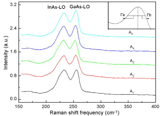
**Fig. 2.** Raman spectrum of  $\text{In}_{0.82}\text{Ga}_{0.18}\text{As}$  epilayer with buffer layer thermal annealing for 0, 2, 5, 10, and 15 min, respectively. The inset shows  $\Gamma_a$  and  $\Gamma_b$  which is used in asymmetry ratio ( $\Gamma_a/\Gamma_b$ ) of Raman scattering spectra.
