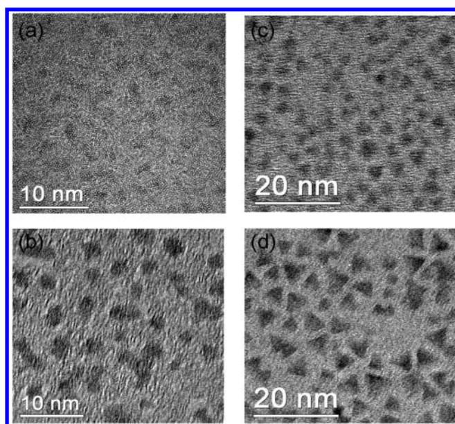
**Figure 2.** TEM images of bare CuInS<sub>2</sub> cores with 2.0 (a) and 3.6 nm (b) diameters and the corresponding CuInS<sub>2</sub>/CdS core/shell QDs (c and d).
