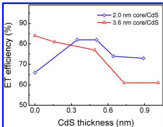
**Figure 7.** ET efficiencies of CuInS<sub>2</sub>/CdS core/shell QDs with core diameters of 2.0 (blue squares) and 3.6 nm (red triangles) and different CdS shell thicknesses attached to TiO<sub>2</sub> films.
