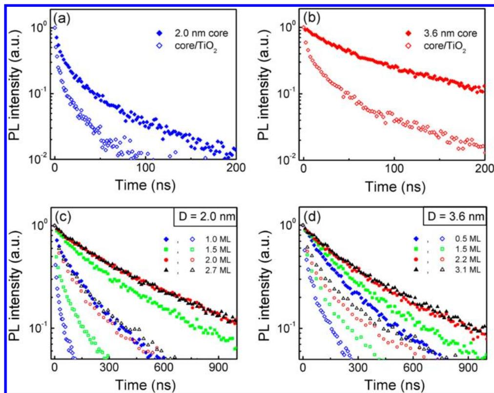
**Figure 4.** PL decay curves of 2.0 (a) and 3.6 nm (b) CuInS<sub>2</sub> core QDs and the corresponding CuInS<sub>2</sub>/CdS core/shell QDs with 2.0 (c) and 3.6 nm (d) core diameters and various CdS shell thicknesses deposited on the TiO<sub>2</sub> (empty symbols) and SiO<sub>2</sub> (solid symbols) films.
