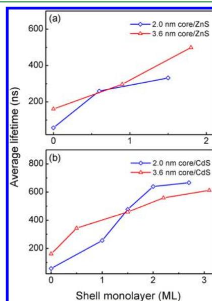
**Figure 3.** Average PL lifetimes of CuInS<sub>2</sub>/ZnS (a) and CuInS<sub>2</sub>/CdS (b) core/shell QDs with 2.0 (blue squares) and 3.6 nm (red triangles) core diameters and different shell thicknesses in toluene.
