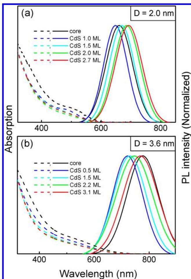
**Figure 1.** UV-visible absorption (dashed lines) and normalized PL (solid lines) spectra of 2.0 (a) and 3.6 nm (b) CuInS<sub>2</sub> core and CuInS<sub>2</sub>/CdS core/shell QDs.
