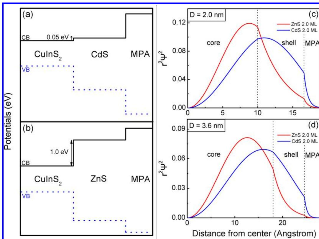
**Figure 6.** Schematic illustration of the band level alignment for CuInS<sub>2</sub>/CdS (a) and CuInS<sub>2</sub>/ZnS (b) core/shell QDs and the radial distribution functions of lowest energy conduction band electrons of CuInS<sub>2</sub>/CdS (blue lines) and CuInS<sub>2</sub>/ZnS (red lines) core/shell QDs with 2.0 (c) and 3.6 nm (d) core diameters and 2.0 ML shell.
