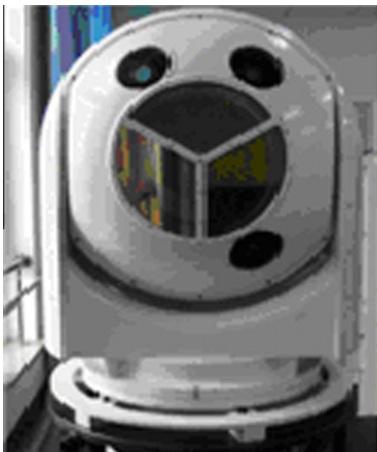
Fig. 1. Prototype of the optical transmitter and receiver with \phi 600 mm.
