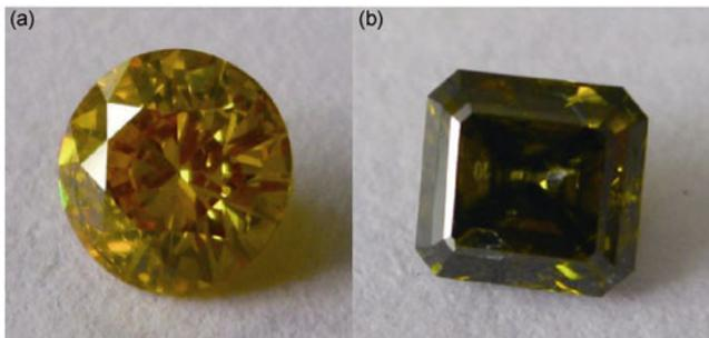
**Figure 3** Optical photos of cut and polished diamond crystals. (a) Type-Ib diamond; (b) boron-doped diamond.
