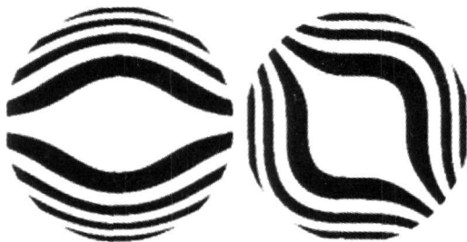
(a) 彗差波面干涉图 (b) 三次位相波面干涉图 (a) the interferogram of coma wavefront (b) the interferogram of cubic wavefront
