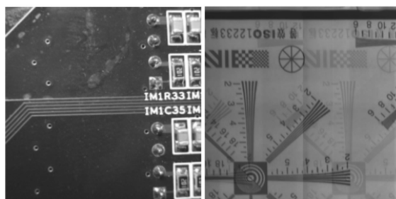
(a) 成像电路PCB (b) 串扰图像 (a) PCB of imaging circuit (b) Crosstalk image
