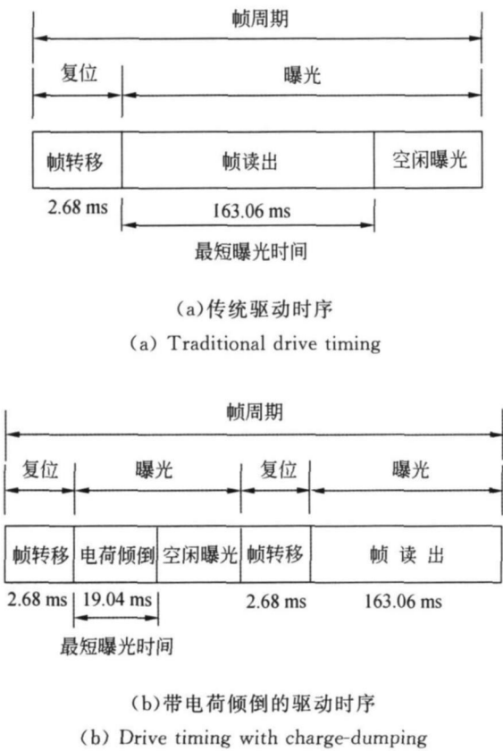
Fig. 5 Diagram of frame-transfer CCD drive timing
