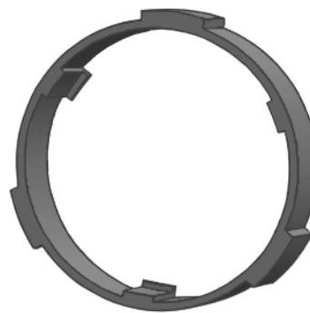
Fig. 5 3-D model of lens radial support structure
