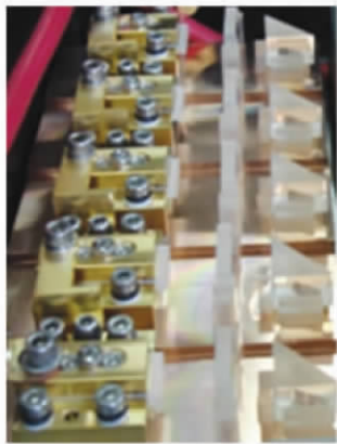
Fig. 2 Mechanical setup of 5 bars mounted in a stair-step manner
