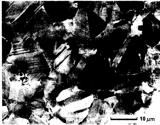
Fig. 3 SEM images showing the surface morphology of the pure nickel samples after the ten-pulse HCPEB irradiation with an accelerating voltage of 21.6 kV
