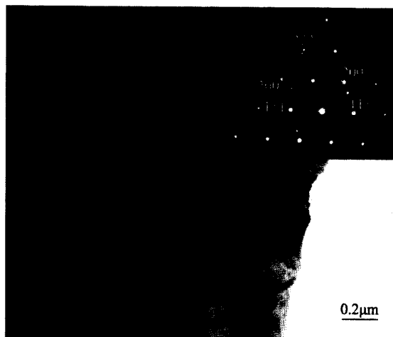
Fig. 5 TEM image of the micro-twins and the corresponding SAED pattern after a five-pulse HCPEB irradiation
