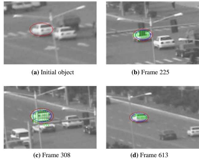
Notes: The “+” (green) indicates the initial positions of mean-shift tracker; the red ellipse (object) and blue ellipse (template) show the tracking result
