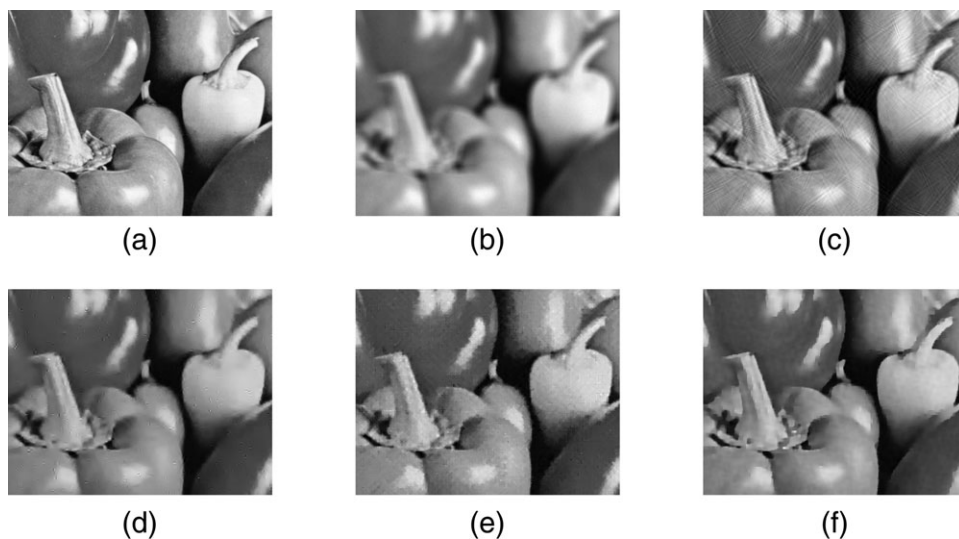
Figure 7. Details of the image deconvolution experiment with a 512 \times 512 Peppers image. (a) Original image. (b) Noisy blurred image, BSNR = 30 dB. (c) ForCuRD estimate, ISNR = 4.53 dB. (d) ForWaRD estimate, ISNR = 3.91 dB. (e) LPA-ICI estimate, ISNR = 4.17 dB. (f) Our method estimate, ISNR = 5.65 dB.
