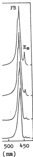
PL spectra at 77 K from ZnSe epilayers grown with B series source materials, excited by the 365.0 nm Hg lamp.
