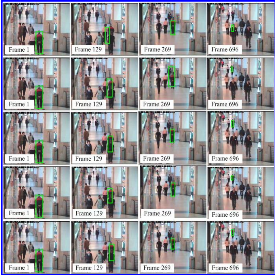
Fig. 6. Covariance tracking for OneStopMoveEnterIcor sequence with random sampling. First row: only 10 random samples are picked from each of the candidate and model images, 20 samples in the second row, 50 samples in the third row, 100 samples in the fourth row and full samples in the last row.
