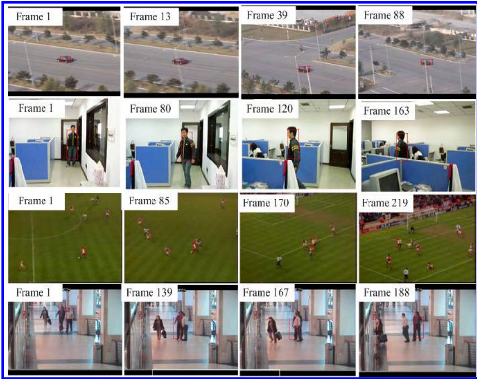
Fig. 2. The test results of proposed method in four different sequences. In the Black Car sequence, the scale and appearance of the object change over time due to the moving camera and object. In the Lab , Soccer and OneShopOneWait2cor sequences, the objects are non-rigid. The appearances of the target change drastically in the Lab sequence. The object is blocked in the OneShopOneWait2cor sequence.
