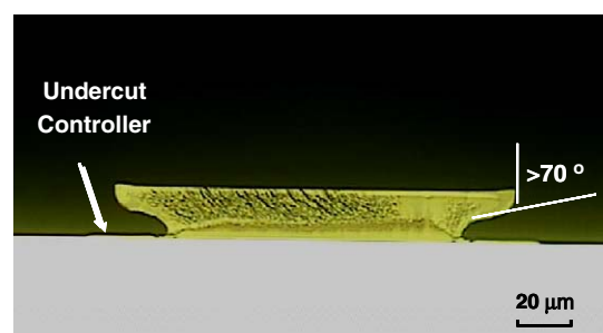
Fig. 3. Micrographic image of pillar cross-section with large undercut and overhang made by the new fabrication method.
