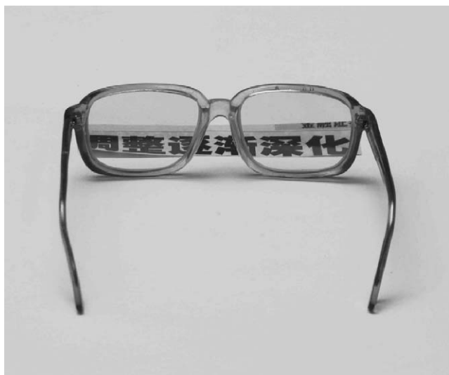
Fig. 7. Photo of the designed eye-protection glasses against YAG laser based on the one-dimensional photonic crystal.
