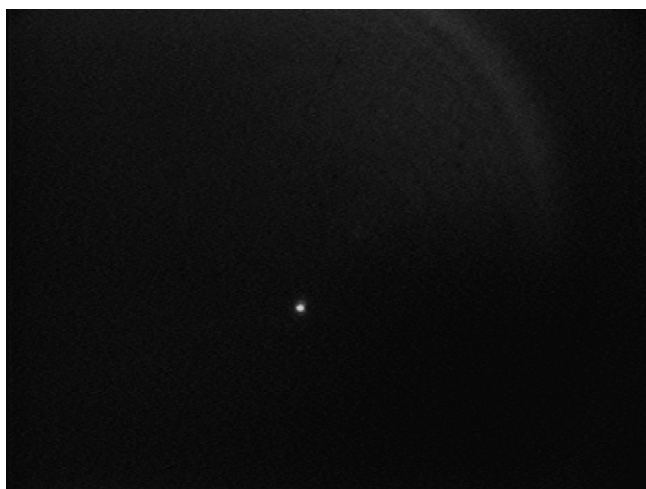
Fig. 5. The output near-field mode profile from a 3.0 cm long waveguide at 1535 nm wavelength.
