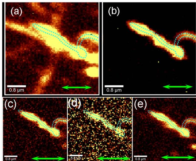
FIG. 2. (Color online) Raman images constructed using peak intensity of (a) *G* band of CNTs, (b) band I of Si-C at  $1510\text{ cm}^{-1}$ , (c) band II of Si-C at  $1692\text{ cm}^{-1}$ , (d) band III at  $2392\text{ cm}^{-1}$ , and (e) band IV at  $2620\text{ cm}^{-1}$ . The green arrow indicates the polarization of the incident laser. The blue dotted curves indicate the position and shape of the special CNT.
