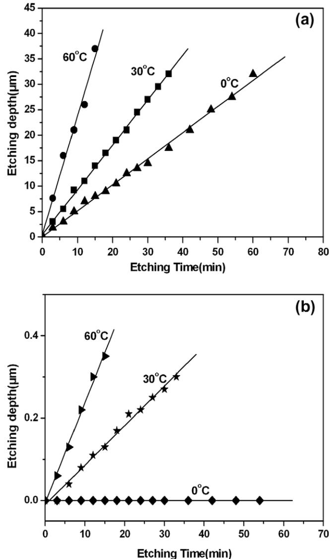
Fig. 4. The dependences of the etching depth on etching time for Al<sub>0.7</sub>Ga<sub>0.3</sub>As and GaAs by concentrated HCl at different temperatures.
