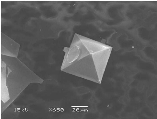
Fig. 5. A SEM image of a removed GaAs microtip.
