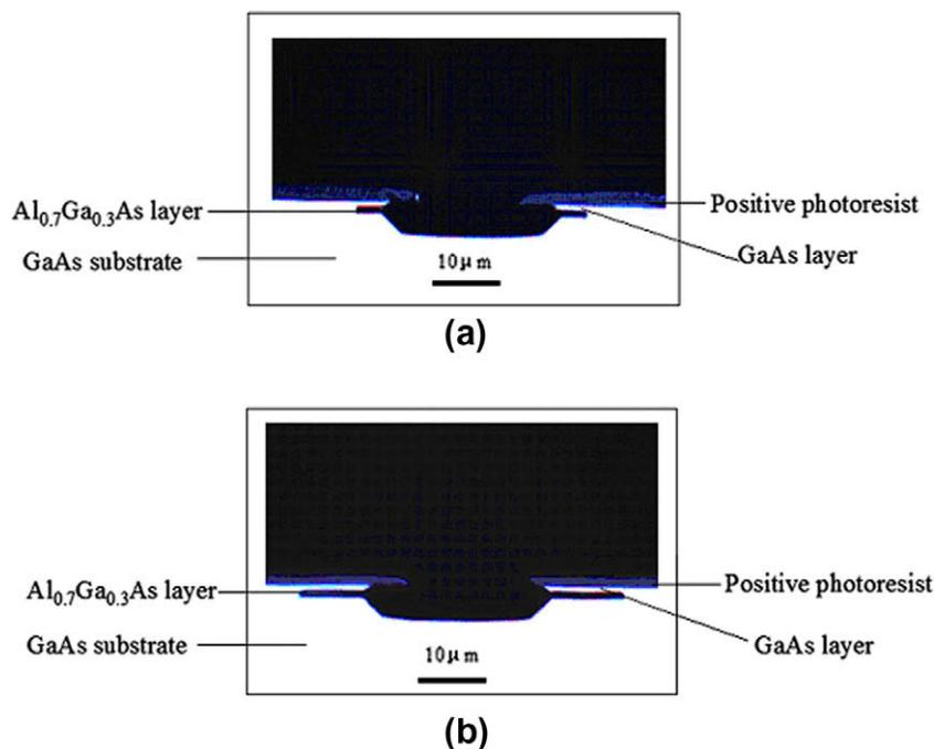
**Fig. 2.** The cross-sectional images of the sandwich structure etched by a 188 solution for 35 s and then etched by a concentrated HCl etchant at 0 °C, (a) for 6 min and (b) for 15 min.
