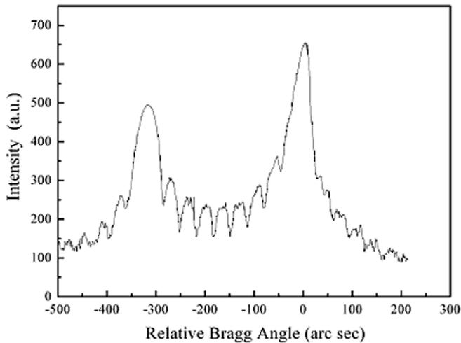
**Fig. 1.** The DCXRD profile of the GaAs/Al<sub>0.7</sub>Ga<sub>0.3</sub>As/GaAs sandwich structure for (0 0 4) plane.
