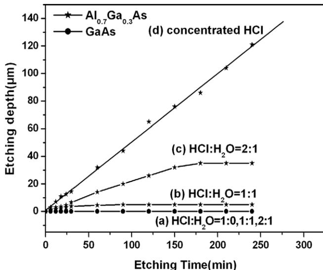
Fig. 3. The dependences of the etching depth on etching time for Al<sub>0.7</sub>Ga<sub>0.3</sub>As and GaAs by different HCl concentrations at 0 °C, (a) HCl:H<sub>2</sub>O = 1:0, 1:1, 2:1 etching of GaAs, (b) HCl:H<sub>2</sub>O = 1:1 etching of Al<sub>0.7</sub>Ga<sub>0.3</sub>As, (c) HCl:H<sub>2</sub>O = 2:1 etching of Al<sub>0.7</sub>Ga<sub>0.3</sub>As and (d) concentrated HCl etching of Al<sub>0.7</sub>Ga<sub>0.3</sub>As.
