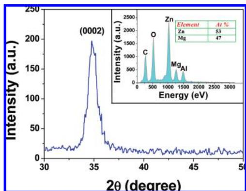
FIGURE 1. XRD spectra of the  $\text{Mg}_{0.47}\text{Zn}_{0.53}\text{O}$  thin film grown on quartz prepared by RF magnetron sputtering. The inset is the EDS spectrum of the  $\text{Mg}_{0.47}\text{Zn}_{0.53}\text{O}$  film.
