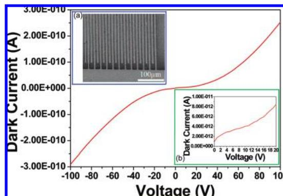
FIGURE 3.  $I$ - $V$  characteristics of the  $\text{Mg}_{0.47}\text{Zn}_{0.53}\text{O}$ -based MSM photodetector. Inset a is the optical microscopic top view of the MSM-structured photodetector showing interdigitated electrodes. Inset b is the  $I$ - $V$  characteristics of the  $\text{Mg}_{0.47}\text{Zn}_{0.53}\text{O}$ -based MSM photodetector on a small voltage scale.
