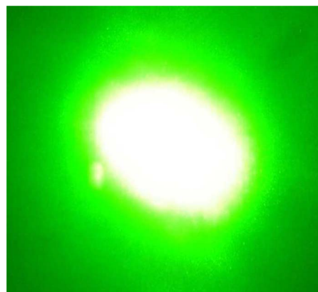
Fig. 6. (Color online) Beam spot of the 556 nm yellow-green laser.
