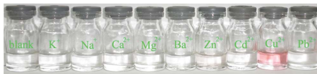
Fig. 4 Change in color of Rh1 (10 \mu\text{M} ) in buffered (NaAc-HAc, pH = 7) water/ \text{CH}_3\text{CN} (1 : 1, v/v) with metal ions: blank, \text{K}^+ , \text{Na}^+ , \text{Ca}^{2+} , \text{Mg}^{2+} , \text{Ba}^{2+} , \text{Zn}^{2+} , \text{Cd}^{2+} , \text{Cu}^{2+} and \text{Pb}^{2+} ( 1 \times 10^{-3} M, from left to right).
