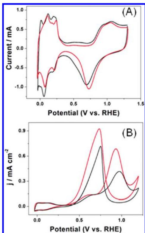
**Figure 4.** Cyclic voltammograms of Pt octahedrons (red) and commercial Pt/C (black) in 0.5 M H<sub>2</sub>SO<sub>4</sub> (A) and 0.5 M H<sub>2</sub>SO<sub>4</sub> + 0.5 M MeOH (B). Scan rate: 100 mV/s.
