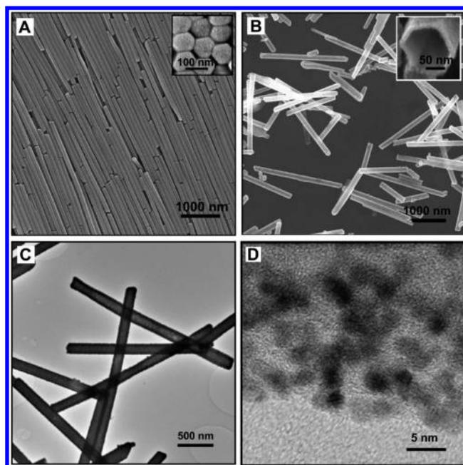
**Figure 1.** Electron microscopy images of the ZnTPyP long wires and the hollow Pt nanotubes. (A) SEM image of ZnTPyP long wires that have hexagonal shape for cross-sectional view. (B) SEM images of Pt nanotubes; inset, high-resolution SEM image shows the hexagonal shape of nanotube. (C) TEM image of Pt nanotubes. (D) Corresponding high-resolution TEM image shows the interconnected Pt network.
