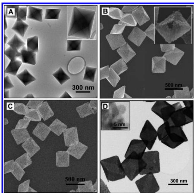
**Figure 2.** (A) TEM image of octahedral ZnTPyP nanocrystals. (B) SEM images of hollow Pt octahedrons; inset, high-resolution SEM image of one chipped specimen showing the hollow cavity. (C) Corresponding backscattering SEM image. (D) TEM image of hollow Pt octahedrons; inset, high-resolution TEM image shows the interconnected Pt particle network.
