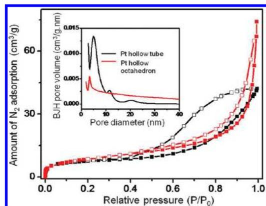
**Figure 3.** Nitrogen sorption isotherms obtained at 77 K for different hollow Pt nanostructures: nanotube (diameter  $\sim$ 150 nm, thickness 15 nm), octahedron (diameter 280 nm, thickness 10 nm): adsorption, solid data markers; desorption, open data markers; inset, pore size distributions for different Pt hollow nanostructures.
