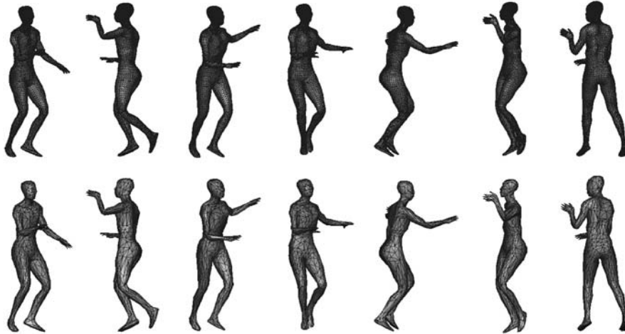
Figure 2 Dancer animation models with 48 frames. Upper row: original sequence with 7061 vertices. Bottom row: simplified models with 700 vertices (remove 90%).
