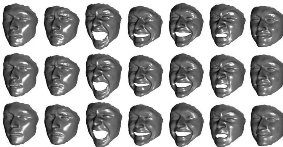
Figure 8 A face-expression animation with 192 frames. Top: The original sequence with 23725 vertices and 46853 faces. Middle: 3201-vertices and 5825-faces approximation (80% reduced). Bottom: 1200-vertices and 1874-faces approximation (95% reduced).
