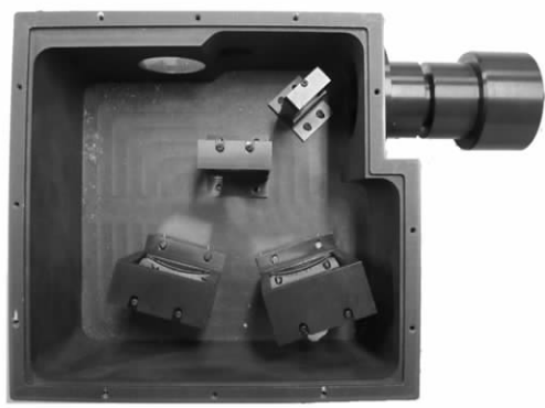
Fig. 9 Imaging spectrometer with convex grating
