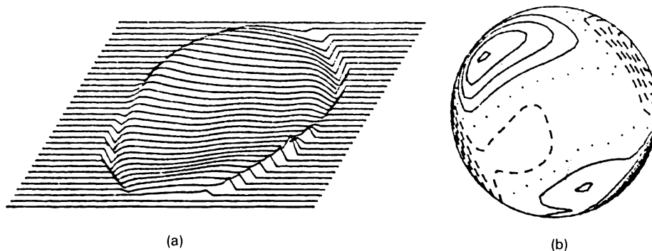
Fig. 4 (a) The 3-D plots and (b) contour of the surface error W_1(x,y) of the large convex spherical surface being tested; PV = 0.59 W, rms = 0.006 W, contour step = 0.05 W.
