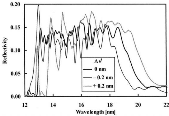
Fig. 6. The calculated reflectivities of Mo/Si depth-graded multilayers designed for flat responses in the wavelength range 13–19 nm, showing the effect of systematic boundary position errors.
