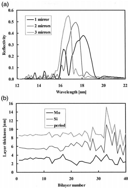
Fig. 2. (a) Calculated optimum normal incidence reflectivities versus wavelength of depth-graded Mo/Si multilayers for different merit functions (integrated reflectivity for 1, 2 and 3 mirrors) in the wavelength range 16–19 nm, and with 0.3 nm interfacial roughness. (b) Layer thicknesses versus the number of bilayers for 3 mirrors.
