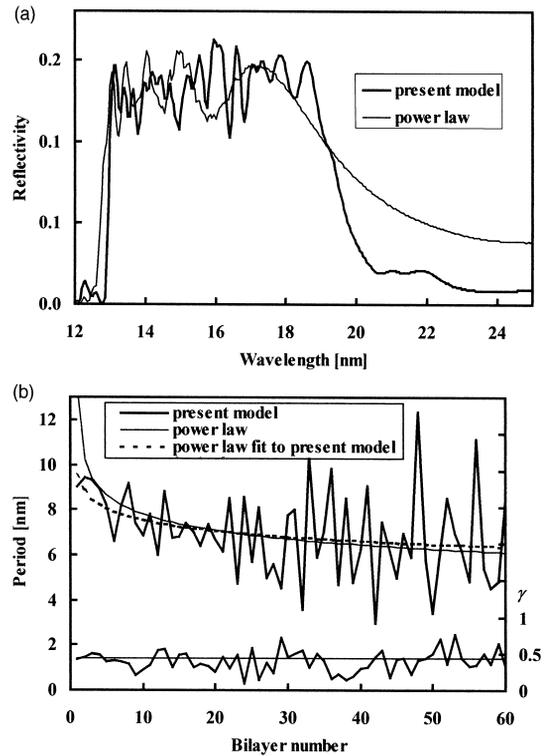
Fig. 9. (a) The calculated reflectivity of the Mo/Si depth-graded multilayer designed for flat responses in the wavelength range 13–19 nm compared to that calculated assuming a power law distribution of bilayer thicknesses. (b) The distribution of bilayer thicknesses in both cases. The lower two curves show the values of  $\gamma$  resulting from the calculations.
