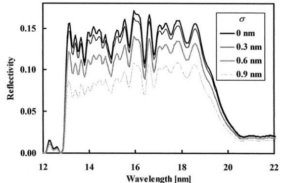
Fig. 5. The calculated reflectivities of Mo/Si depth-graded multilayers designed for flat responses in the wavelength range 13–19 nm, showing the effect of roughness.
