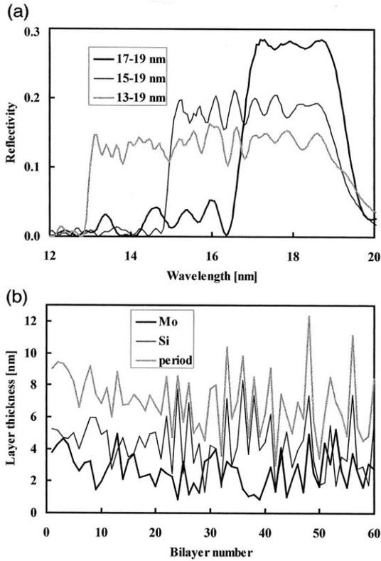
Fig. 4. (a) Calculated reflectivities of three depth-graded Mo/Si multilayers designed for flat responses in three different wavelength intervals. (b) Layer thickness distributions for the wavelength range 13–19 nm.
