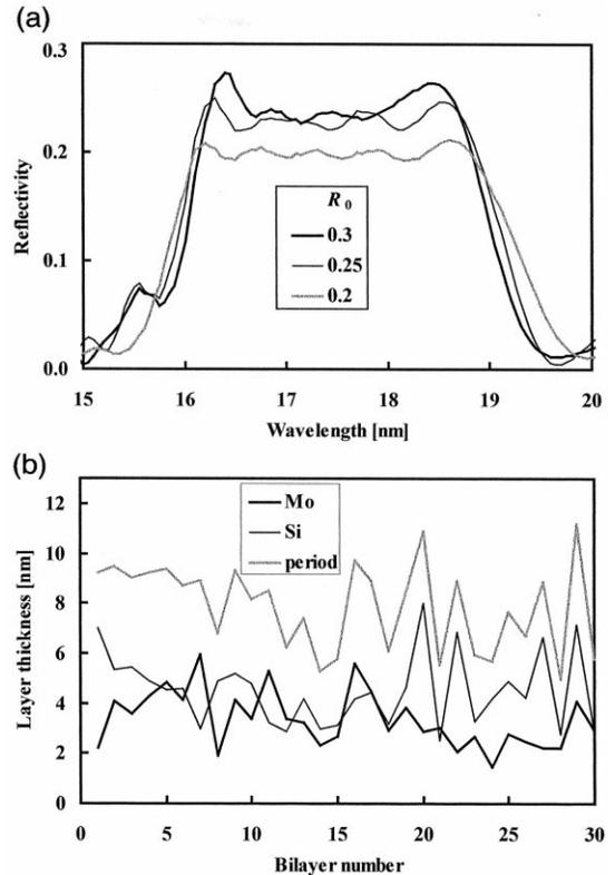
Fig. 3. (a) Calculated optimum reflectivity versus wavelength using the merit function to give a flat response with different target reflectivities, assuming 0.3 nm interfacial roughness. (b) Layer thicknesses of layers as a function of the bilayer number for a target reflectivities of 0.2.
