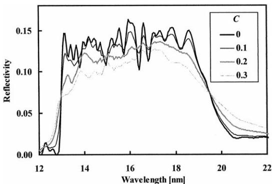
Fig. 7. The averaged calculated reflectivities of Mo/Si depth-graded multilayers designed for flat responses in the wavelength range 13–19 nm, showing the effect of random boundary position errors.
