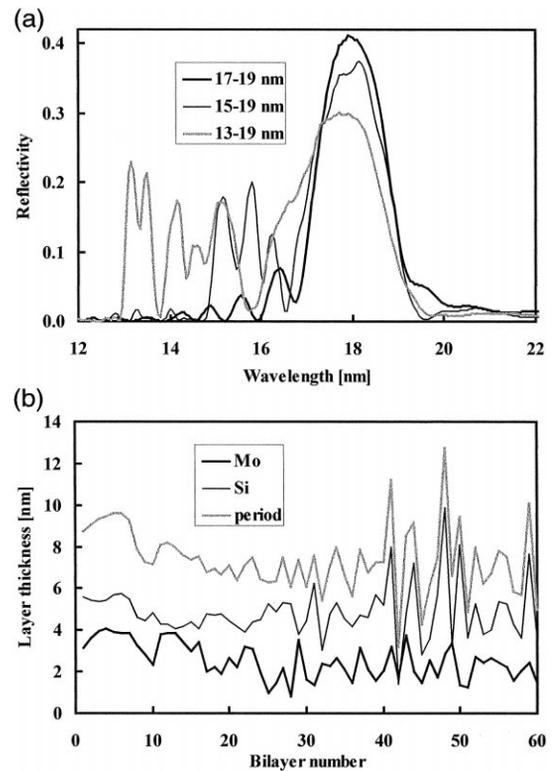
Fig. 1. (a) Calculated optimum normal incidence reflectivities versus wavelength of depth-graded Mo/Si multilayers for different wavelength ranges. The merit function to optimise the integrated reflectivity for one mirror was used, and an interfacial roughness of 0.3 nm was assumed. (b) Layer thicknesses versus the number of bilayers for the wavelength range 13–19 nm.
