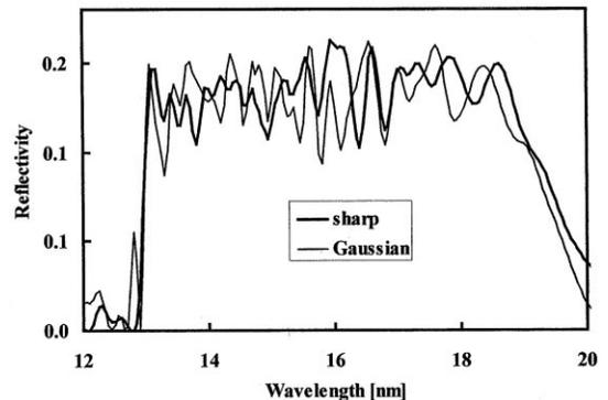
Fig. 8. The calculated reflectivities of Mo/Si depth-graded multilayers designed for flat responses in the wavelength range 13–19 nm, showing the effect of non-sharp boundaries.
