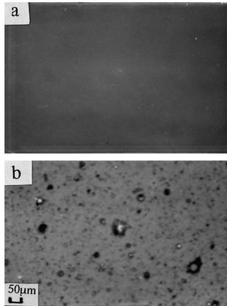
Fig. 3. Microscopic images that show debris adhered on the surface of witness plates. (a) CO<sub>2</sub> cryogenic target, (b) Cu target.
