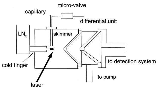
Fig. 1. Schematic of the cryogenic target chamber.
