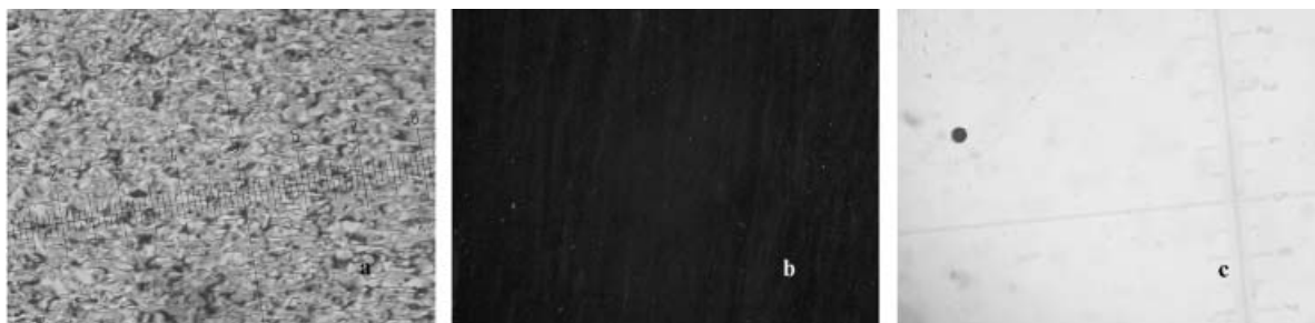
Figure 8. Photomicrographs of a liquid crystal cell under polarizing microscopy: (a) liquid crystal cell with un-irradiated 6 bi-layer LBL multilayer film (random alignment); (b) parallel cell with photoalignment film irradiated 5 min with polarizers parallel to the optical axis of the sample (planer alignment); (c) parallel cell with irradiated film with polarizers at 45° to the optical axis of the sample.
