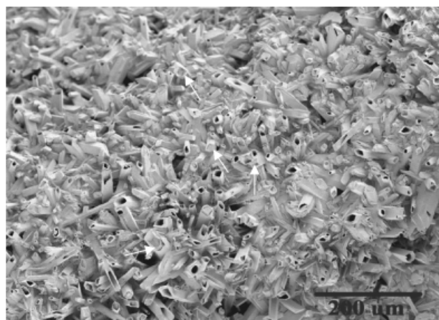
Fig. 3. Scanning electron microscopy micrograph of \text{Al}_{18}\text{B}_4\text{O}_{33} microtubes synthesized via simply high-temperature calcining the mixture of aluminum and boron nitride at 1700^\circ\text{C} for 2 h.
