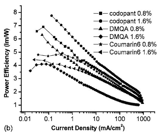
FIG. 3. (b) the power efficiency vs current density characteristics
