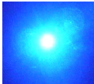
Fig. 7. The beam shape of 457 nm blue laser. (For interpretation of the references to color in this figure legend, the reader is referred to the web version of this article.)
