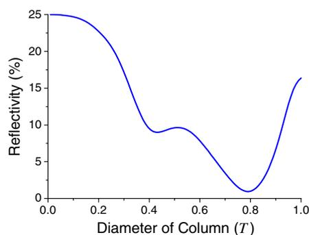
**Figure 5.** Relation between reflectivity and column diameter for a silicon substrate, with parameters:  $T = 0.69\lambda$ ;  $h = 0.16\lambda$ ;  $\psi = 90^\circ$ ;  $\alpha = \delta = 0^\circ$ ;  $n_i = 1.0$ ;  $n_s = 3.0$ ;  $M = N = 13$ .
