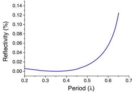
**Figure 8.** Relation between reflectivity and spatial period for a glass grating, with parameters:  $R = 0.79T$ ;  $h = 0.205\lambda$ ;  $\psi = 90^\circ$ ;  $\alpha = \delta = 0^\circ$ ;  $n_i = 1.0$ ;  $n_s = 1.5$ ;  $M = N = 13$ .
