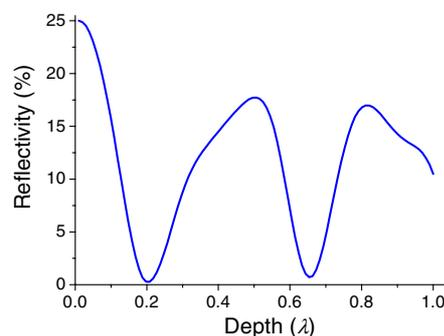
**Figure 7.** Relation between reflectivity and the depth of a silicon grating, with parameters:  $T = 0.69\lambda$ ;  $R = 0.71T$ ;  $\psi = 90^\circ$ ;  $\alpha = \delta = 0^\circ$ ;  $n_i = 1.0$ ;  $n_s = 3.0$ ;  $M = N = 21$ .
