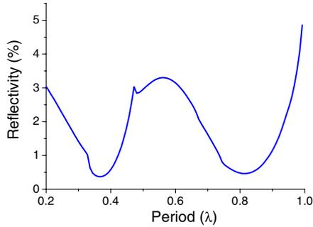
**Figure 9.** Relation between reflectivity and spatial period for a silicon grating, with parameters:  $R = 0.70T$ ;  $h = 0.17\lambda$ ;  $\psi = 90^\circ$ ;  $\alpha = \delta = 0^\circ$ ;  $n_i = 1.0$ ;  $n_s = 3.0$ ;  $M = N = 13$ ;
