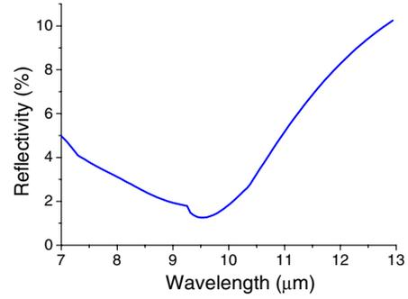
**Figure 13.** Diagram of reflectivity in the far-infrared wave band for a silicon grating, with parameters:  $\lambda_0 = 10 \mu\text{m}$ ;  $T = 0.69\lambda_0$ ;  $R = 0.79T$ ;  $h = 0.15\lambda_0$ ;  $\alpha = \delta = 0^\circ$ ;  $\psi = 90^\circ$ ;  $n_i = 1.0$ ;  $n_s = 3.0$ ;  $M = N = 21$ .
