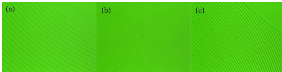
Fig. 4. 200\times magnified images of the fabricated DOEs with the period of 20\mu\text{m} (a), 10\mu\text{m} (b) and 5\mu\text{m} (c) captured by optical microscope.
