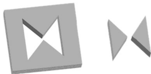
Fig. 3 Schematic of bowtie aperture (left) and antenna (right). Reprinted with permission from [38]
