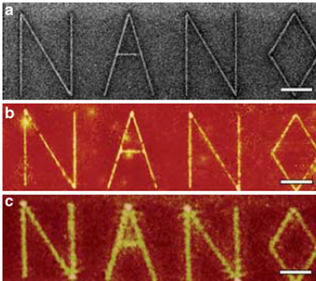
Fig. 9 a FIB image of “NANO” object. b The developed image with silver superlens. c The image in the control experiment. Reprinted with permission from [63]
