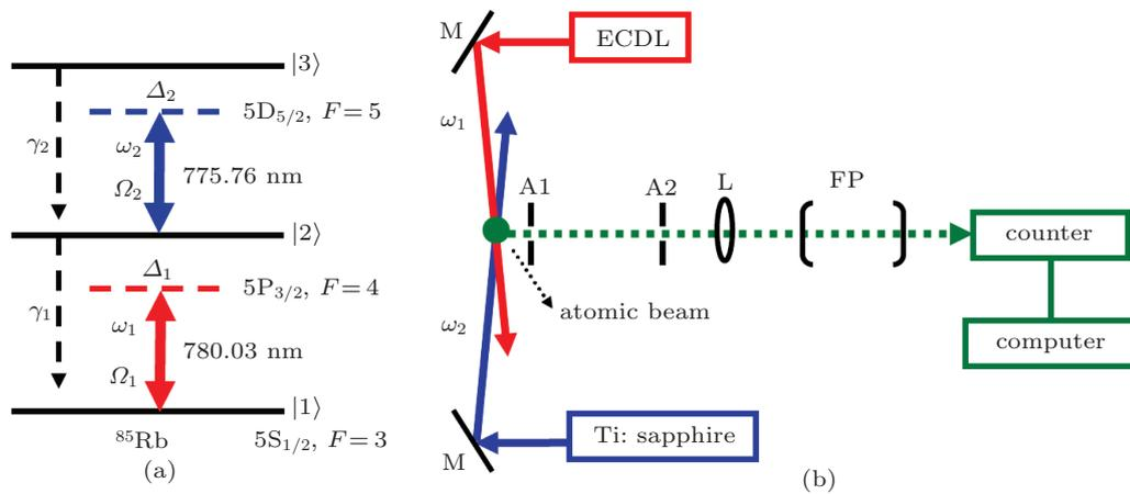
**Fig. 4.** (colour online) (a) Energy-level scheme for  $^{85}\text{Rb}$ . (b) Schematic diagram of the experimental setup, where ECDL stands for external cavity diode laser; Ti:sapphire refers to coherent-899 Ti: sapphire laser; A1 and A2 denote apertures; L represents lens; FP is the Fabry–Perot interferometer.
