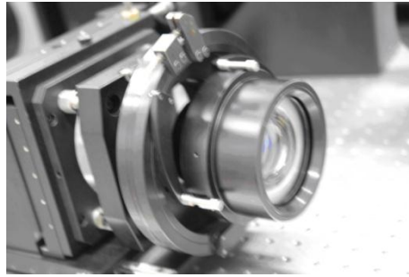
Fig. 13. Photograph of integration of the SACS and the lens enclosed by the test surface.
