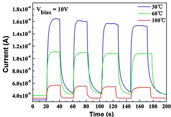
Fig. 5. The photocurrent curves of the ZnO nanowires devices with the 6.5  $\mu\text{m}$  finger distance at 10 V bias at various temperature.
