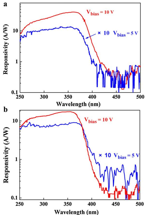
**Fig. 3.** The photoresponsivities of the ZnO nanowires devices with the (a) 6.5  $\mu\text{m}$  and (b) 10  $\mu\text{m}$  finger distance at 5 V and 10 V bias.
