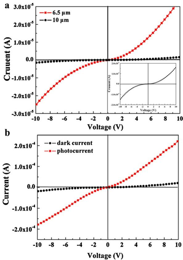
**Fig. 2.** (a) The  $I$ - $V$  curves of the ZnO nanowires devices with the 6.5  $\mu\text{m}$  and 10  $\mu\text{m}$  finger distance (inset is an enlarge image of the  $I$ - $V$  curve with 10  $\mu\text{m}$  finger distance), (b) the photoilluminated  $I$ - $V$  characteristic of the ZnO nanowires devices with the 6.5  $\mu\text{m}$  finger distance.
