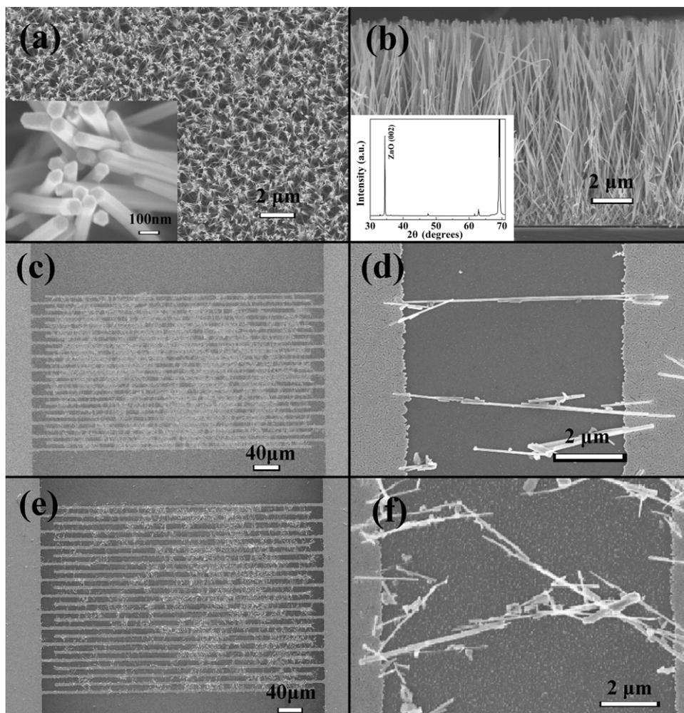
**Fig. 1.** (a) Typical SEM image of ZnO nanowires (inset is a high-magnification image of nanowires), (b) the profile image of ZnO nanowires (inset is the XRD pattern of ZnO nanowires), (c)–(f) shows the SEM images of the ZnO NWs on the Au electrodes with different finger distances arrayed by dielectrophoresis method, the finger distances of (c) and its high-magnification image (d) is 6.5  $\mu\text{m}$ , the finger distances of (e) and its high-magnification image (f) is 10  $\mu\text{m}$ .
