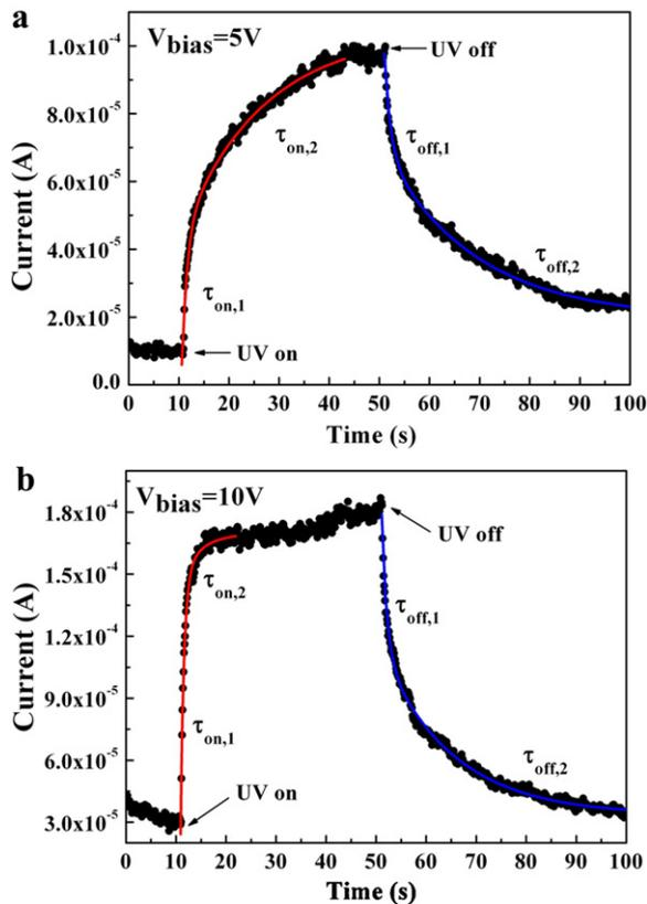
Fig. 4. The decaying and rising of the photocurrent curves and the fitted biexponentially curves of the ZnO nanowires devices with the 6.5  $\mu\text{m}$  finger distance at (a) 5 V and (b) 10 V bias.
