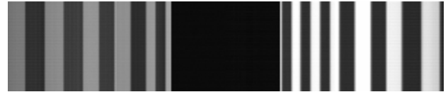
Fig. 12 Test image of eight-channel TDICCD output
